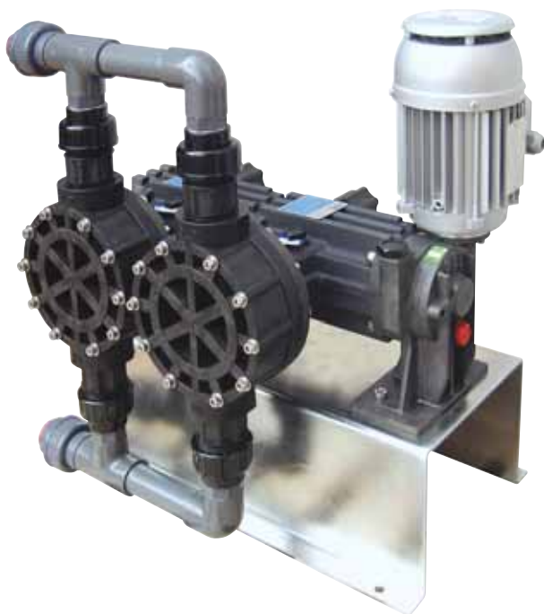
Two-headed MC PP pump head with PVC manifold (1" BSP f threaded connections). Max flow rate 840 l/h, max pressure 5 bar g.
